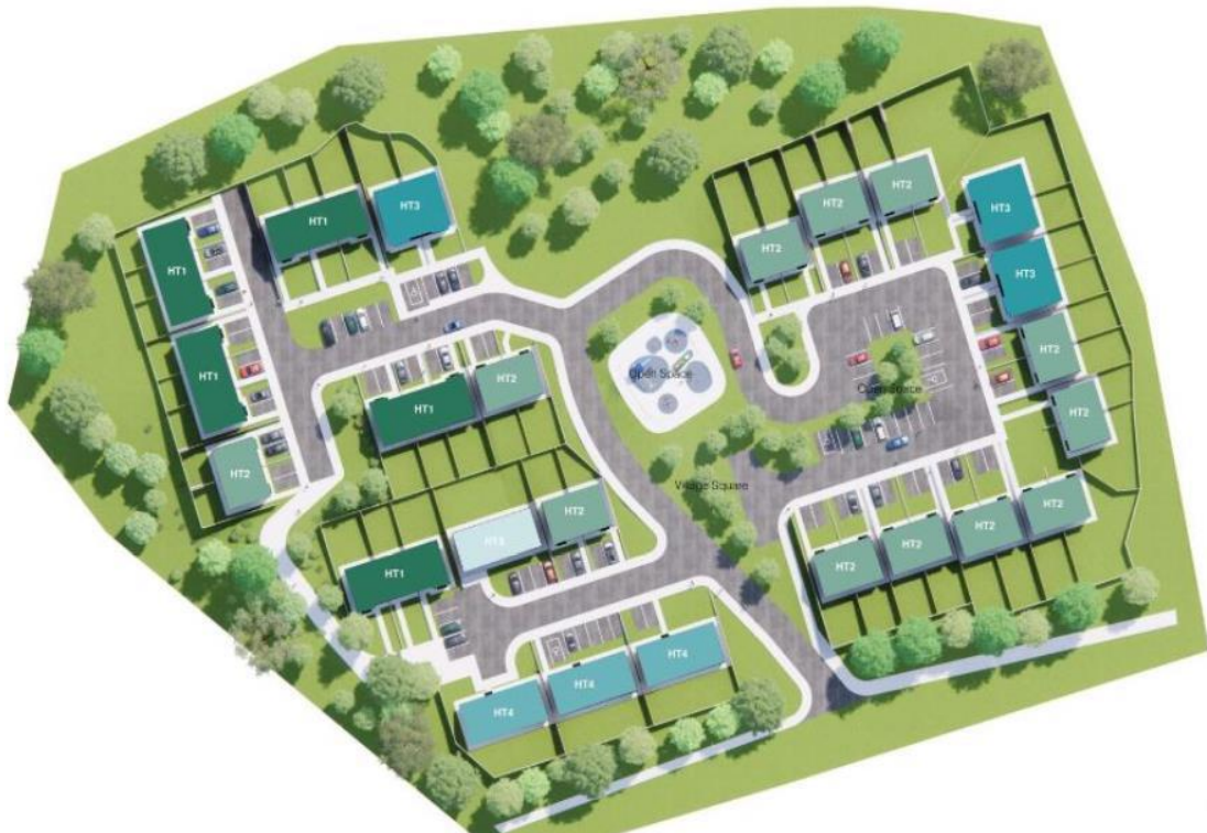
Example of typical Medium B density scheme. Incorporates Semi-detached, terrace and bungalow type houses + some duplex units Density of scheme: approx. 22 units per hectare.
