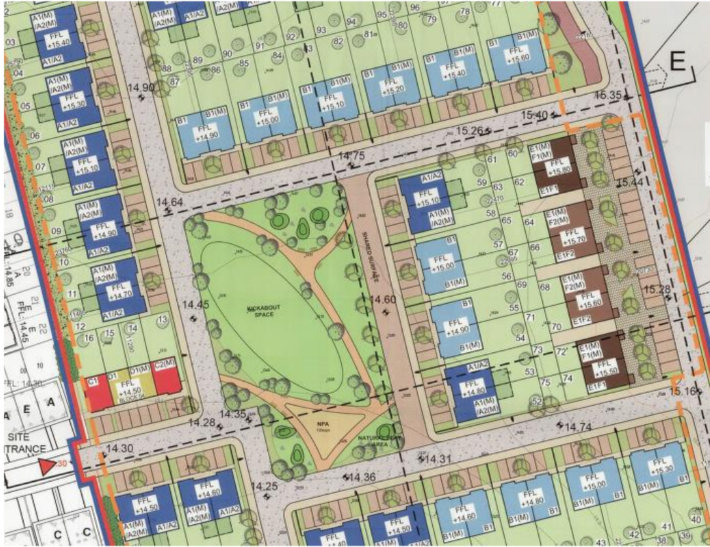
Example of typical Medium A density scheme. Incorporates Semi-detached & terrace type houses + some duplex units for higher density on the eastern side (see image further below) Density of scheme: approx. 36 units per hectare.
